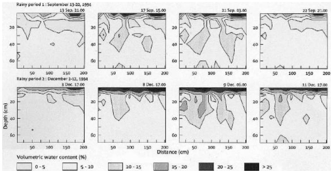
**Figure 2. Spatial distributions of soil water content in the 2 m long and 0.7 m deep TDR trench before, during and after the rainy periods selected.**
