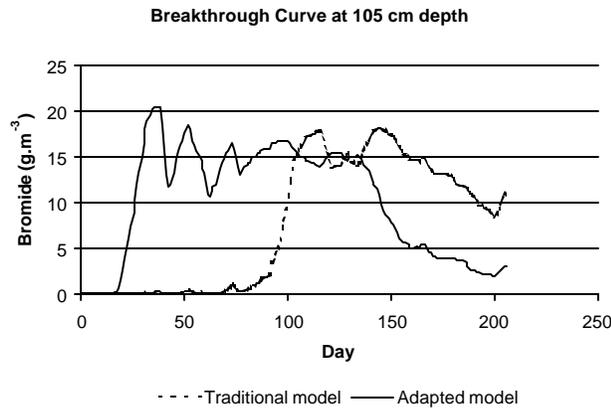
**Figure 4. Breakthrough curves of bromide at 105 cm depth computed with the traditional and adapted SWAP model, i.e. without and with accounting for preferential flow, respectively.**
