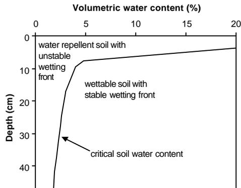
**Figure 1. Critical soil water content versus depth for the Ouddorp soil. In the zone left to the critical soil water contents, the soil is water repellent resulting in the formation of preferential flow paths during infiltration events. At higher soil water contents, the soil is wettable with uniform flow behaviour.**
