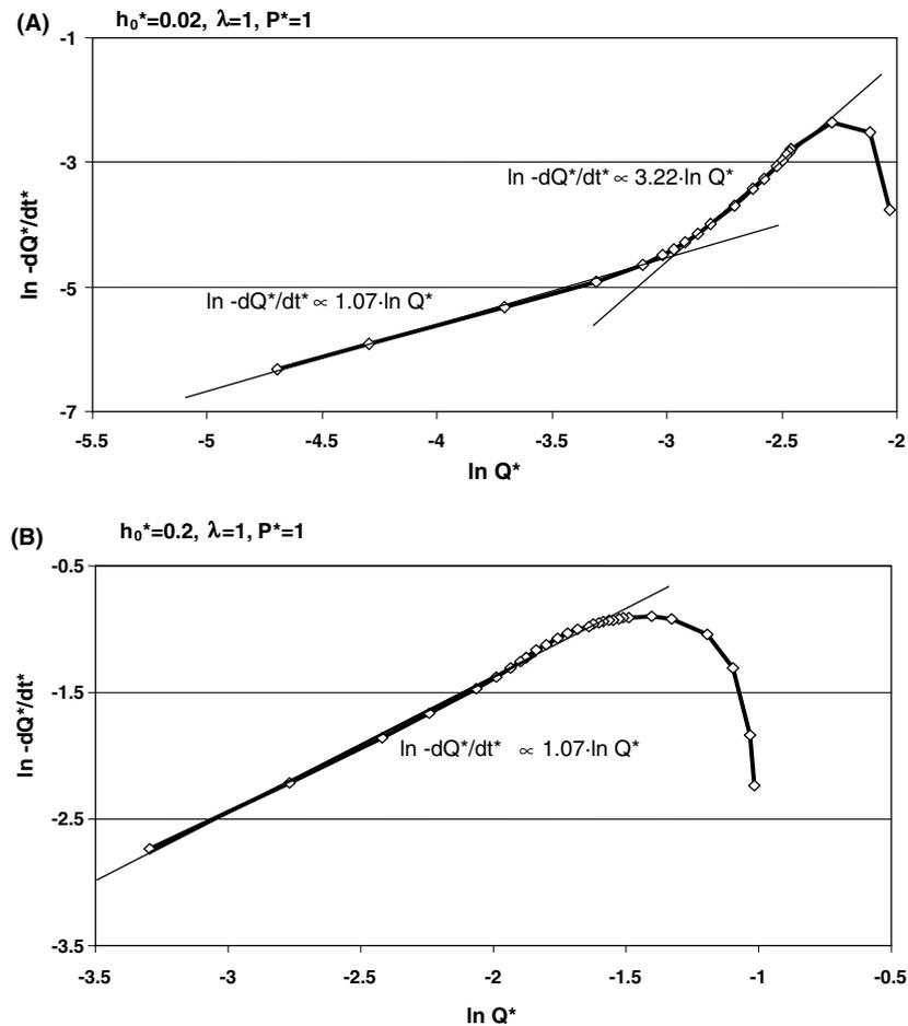
Fig. 4. (A) Recession after cosine-shaped pulse input with  $h_0^* = 0.02$ . (B) As (A) with  $h_0^* = 0.2$ . Formulas refer to thin regression lines that are fitted to (more or less) linear segments. The right side of the curves corresponds to short times, the left side corresponds to long times.
