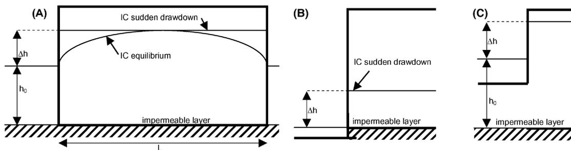
Fig. 1. Geometry and different boundary (BC) and initial conditions (IC) discussed. (A) Drains fully penetrate aquifer, water depth in drains large compared to changes in water table (main geometry discussed). (B) Same as (A) but with zero water height in the drains after drawdown. (C) Same as (A) but with partially penetrating drain.
