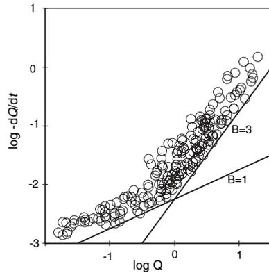
Fig. 2. Sketch of typical results found by Brutsaert and Lopez [2], with  $Q$  and  $t$  in arbitrary units. The fixed lines show the outer envelopes for two values of the exponent  $B$  in Eq. (1).
