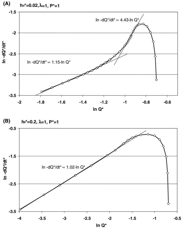
Fig. 5. (A) Recession after equilibrium  $h_0^* = 0.02$ . (B) As (A) with  $h_0^* = 0.02$ . Formulas refer to thin regression lines that are fitted to (more or less) linear segments. The right side of the curves corresponds to short times, the left side corresponds to long times.
