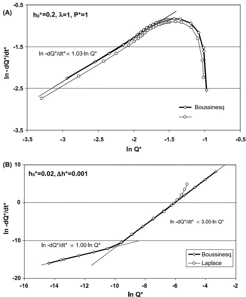
Fig. 6. Comparison of Boussinesq and Laplace solutions. (A) Impulse input. (B) Sudden drawdown. Formulas refer to thin regression lines that are fitted to (more or less) linear segments of the (thick) Boussinesq-based curves. The right side of the curves corresponds to short times, the left side corresponds to long times.
