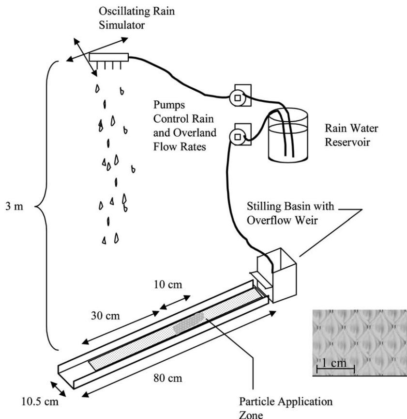
**Figure 2** Schematic of experimental set-up and apparatus. Overland flow can be generated independently of rainfall by spilling water from the stilling basin. Inset is a scale image of the prismatic, polycarbonate diffuser plate used as the roughness surface in the experiments. Indentions are approximately 1 mm deep.
