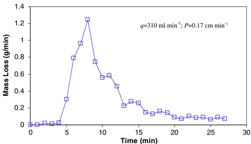
Figure 6 Mass loss curve for surface with deep depressions. The long tail is due to particle detention in the depressions.
