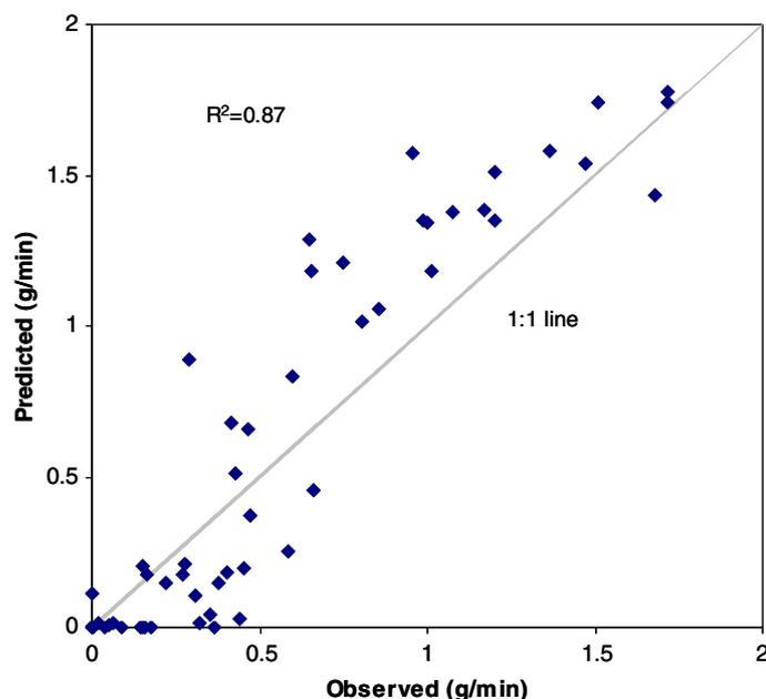
**Figure 5** Comparison of observed versus predicted mass loss values for all runs. Observed values are average of duplicates for each run. Modeled values are the cumulative mass loss over a minute interval – the quantity directly measured in the experiment.
