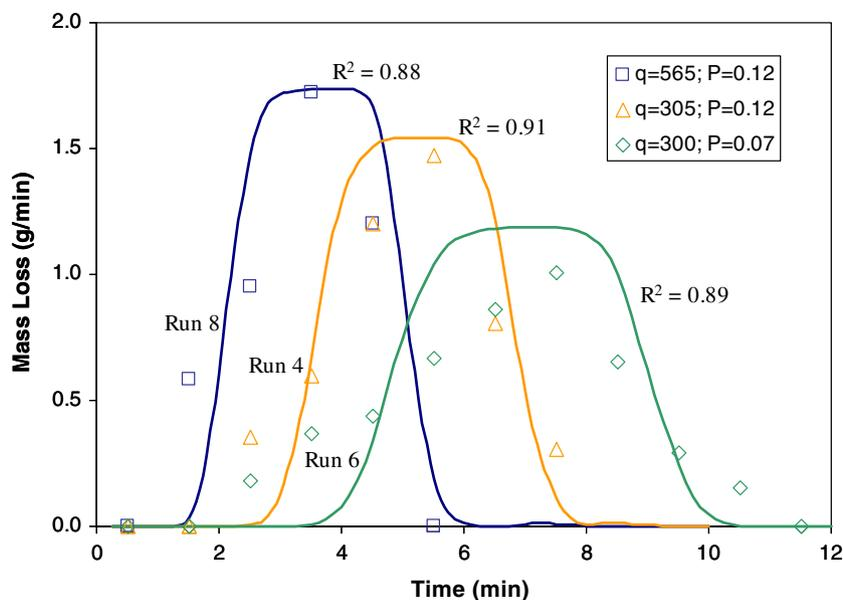
**Figure 4** Model fitted to observed mass loss for experiments with varying rainfall and overland flow rates. Initial  $M_g$  is  $0.05 \text{ g/cm}^2$  for all runs. The rainfall rate ( $P$ ) ( $\text{cm min}^{-1}$ ) and upslope flow rate ( $q$ ) ( $\text{mL min}^{-1}$ ) are indicated. Solid lines are model results while points are observations (squares:  $q = 565/P = 0.12$ ; triangles:  $q = 305/P = 0.12$ ; diamonds:  $q = 300/P = 0.07$ .)
