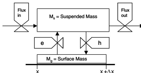
**Figure 1** Flow diagram illustrating interaction between particles in suspension and particles on rough, impervious surface for a distinct control volume. Downslope particle motion occurs only when particles are in motion.
