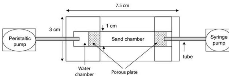
**Figure 3.** Schematic of the unsaturated sand flow chamber.
