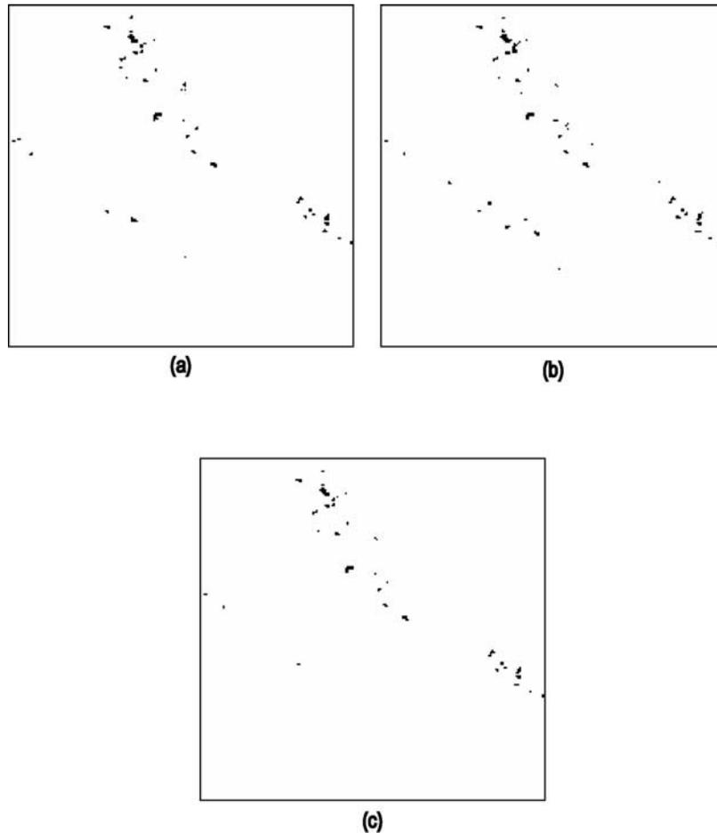
**Figure 5.** Boolean “and” operation: (a and b) two consecutive images with  $\Delta t = 1$  s and (c) pixel remaining at exactly the same position after performing the “and” operation.
