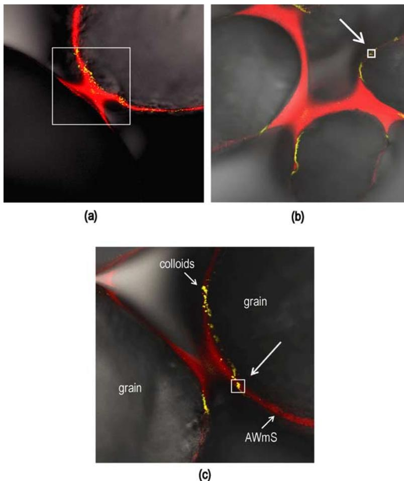
**Figure 2.** Three-channel overlaid confocal scanning laser microscope channel images from (a) series 1 ( $512 \times 512$  pixels,  $748 \times 748 \mu\text{m}$ ), (b) series 2 ( $1024 \times 1024$  pixels,  $748 \times 748 \mu\text{m}$ ), and (c) series 3 ( $512 \times 512$  pixels,  $374 \times 374 \mu\text{m}$ ). The white rectangles in Figures 2a, 2b, and 2c are the locations of enlarged images shown as Figures 4, 7, and 8, respectively.
