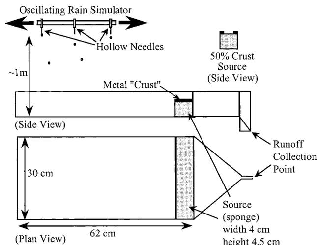
Fig. 2. Experimental flume setup. The flume is metal.
