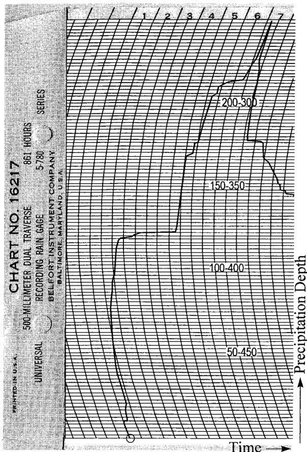
FIG. 1. An example of a portion of a recording, weighing-bucket rain gauge chart (data: Chiloe, Chile).
