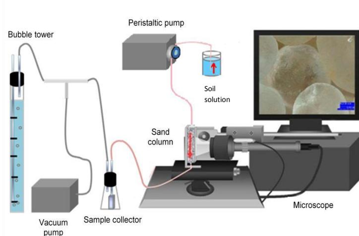
*Figure 2: Illustration of infiltration measurement showing the microscope connected to the camera capturing the vertical movement of soil solution in the column. The peristaltic pump is used to regulate the flow rate into the column and the suction by bubble tower is used to regulate regular leachate collection in the sample collector: Image adapted from Sang (2012).*
