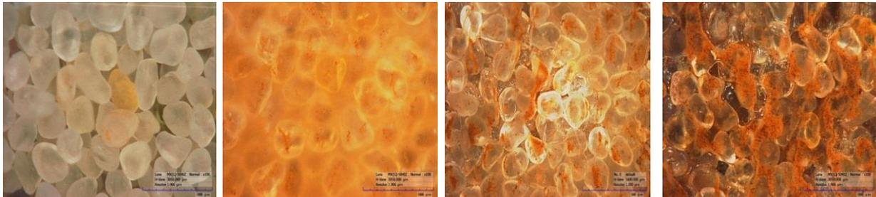
Figure 2: Microscope image of infiltration measurement showing the sand column at the start of the measurement, 30 minutes of soil solution application, 1 hr application and 2 hrs after the second soil solution infiltration on the previous sand column respectively.
