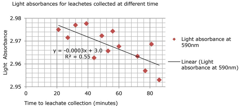
Figure 5: Light absorbance plotted against leachates collection time. The first leachate was collected at the 21st minutes from the beginning of the infiltration measurement.
