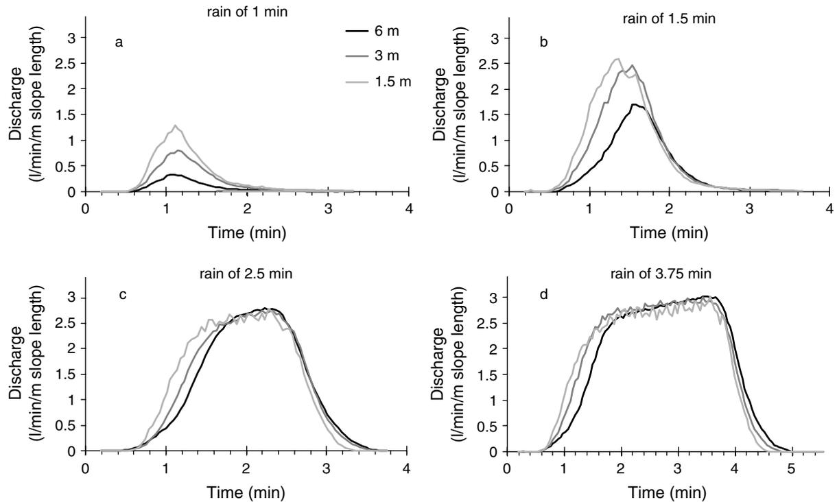
Figure 1. Runoff discharge per unit area ( $1 \text{ min}^{-1} \text{ m}^{-1}$  slope length) from the artificial slope under (a) 1 min, (b) 1.5 min, (c) 2.5 min, and (d) 3.75 min rainfall. The three lines indicate plot lengths of 1.5, 3, and 6 m
