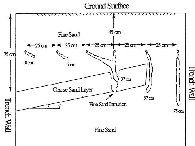
Figure 2. Pattern of dye movement four months after application. Distances below dye plumes indicate maximum vertical movement.
