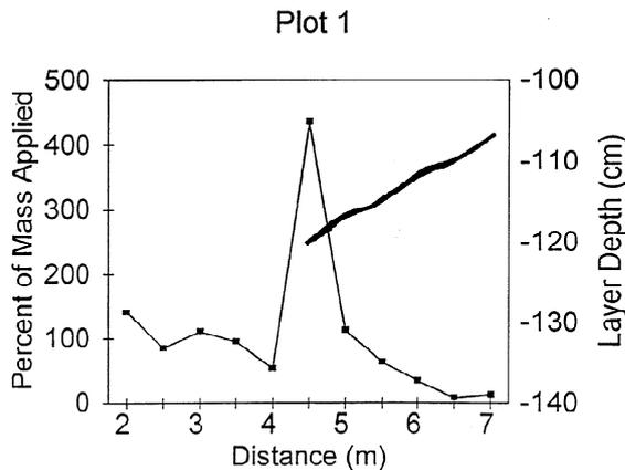
Figure 3. Layer configuration and percent chloride recovered in soil cores in a transect in plot 1. Dark solid line indicates the layer location. Solid squares and line is the percent of the chloride recovered from the application.
