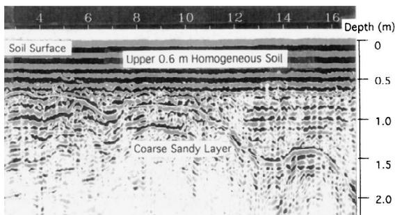
Figure 4. GPR transect for the 1990 nitrate leaching experiment at the South Deerfield site showing the presence of the coarse sandy layer between 0.6 and 1.5 m depth. The sampler is located at left-hand side where the layer is the most shallow.
