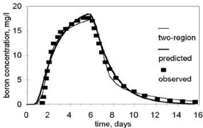
Figure 2. Observed and predicted boron concentration with two-region model (Parker van Genuchten, 1984) and “predicted” with superposition of Eq. (5).
