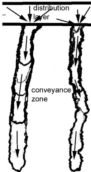
**Figure 1. Schematic for preferential flow.**
