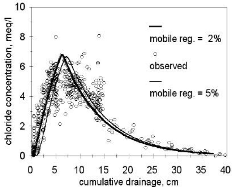
**Figure 3. Observed and predicted breakthrough curves for 39 Arkport sandy loam columns using Eq. (5).**
