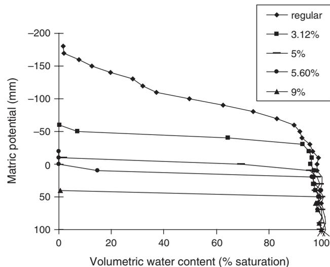
**Fig. 2.** Drying curves for identical sands with different degrees of hydrophobicity.
