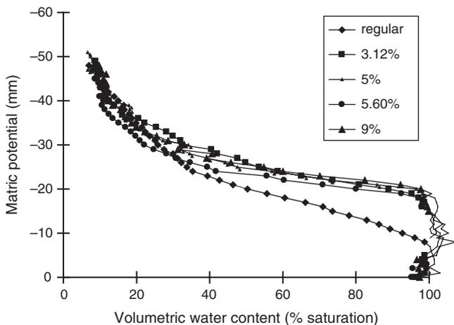
**Fig. 1.** Wetting curves for identical sands with different degrees of hydrophobicity.
