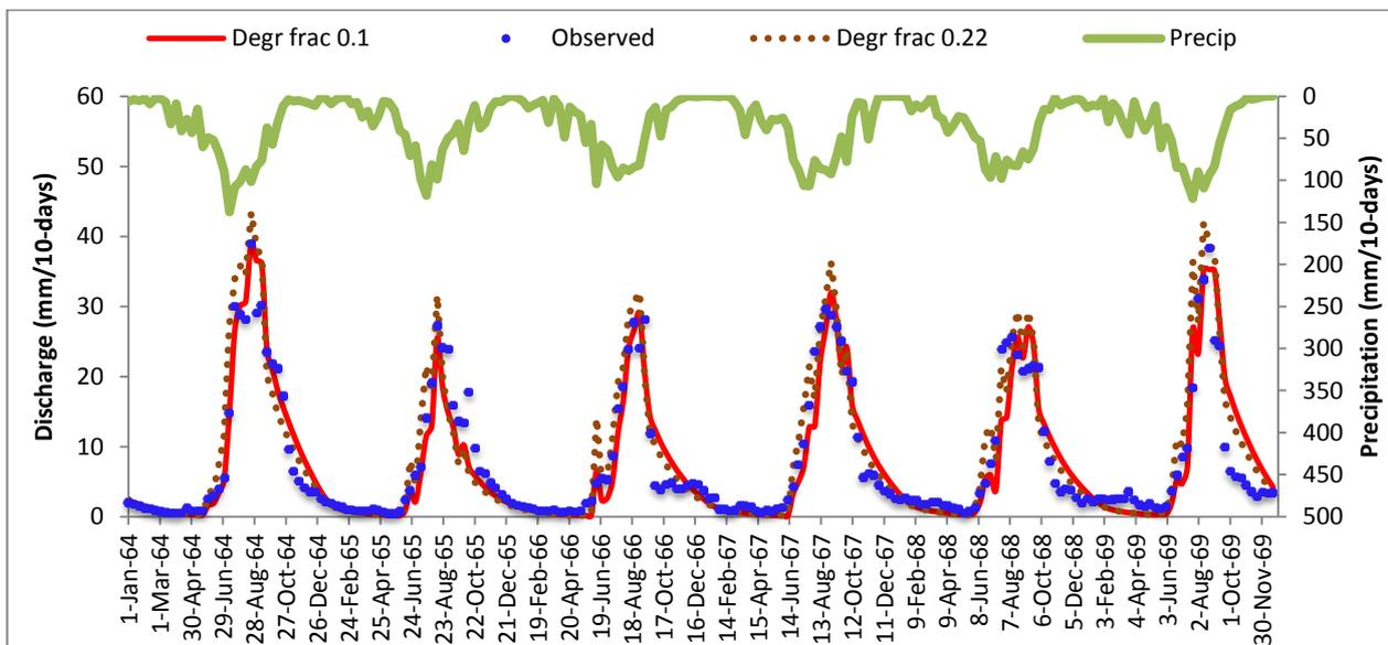
Figure 3: Observed (closed spheres) and predicted (solid line, with 10% of the watershed consist of degraded hillslopes) discharge for the Blue Nile at El Diem at the Ethiopian Sudan border for the period of 1963 to 1969. The dotted line is the discharge assuming that the degraded areas constitute 22% of the landscape.
