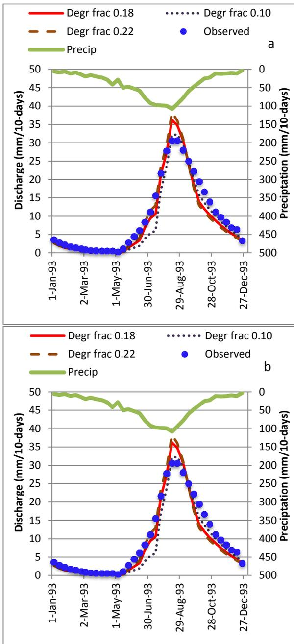
Figure 4: Observed (closed spheres) and predicted discharge (solid line) for 1993 for the Blue Nile at El Diem at the Ethiopian Sudan border where 18% of the watershed consist of degraded hillsides (top figure, a) and lower figure b for 2003 where the solid line represents 22% of the watershed is degraded. The dotted line represents the discharge when the watershed has 10% degraded area and the dashed line the 22% degraded area in a) and 18% b).
