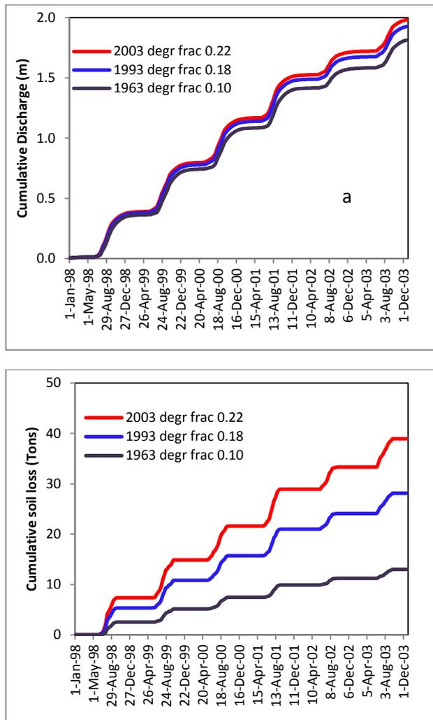
Figure 6: Cumulative runoff (a) and sediment losses (b) for the Blue Nile at the border with Sudan for the period 1998-1993 assuming an increasing fraction of the land landscape becoming degraded
