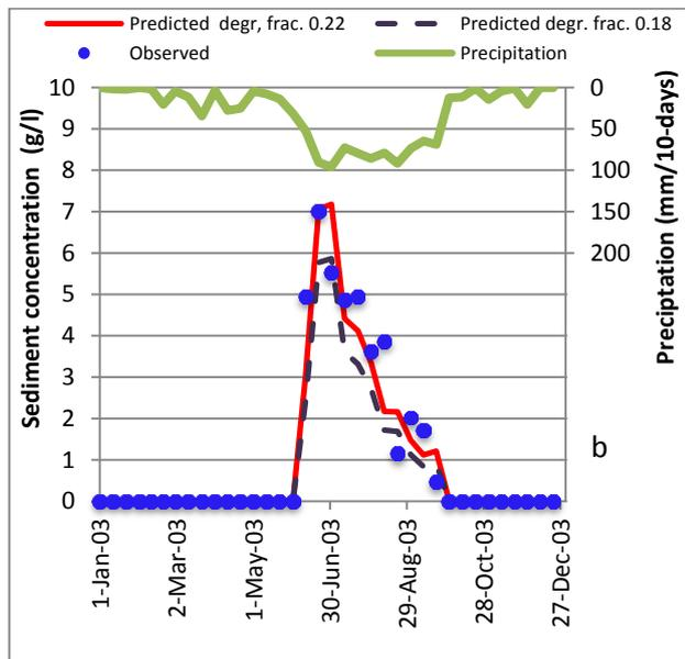
Figure 5: Observed (closed spheres) and predicted sediment concentrations (solid line) for 1993 for the Blue Nile at El Diem at the Ethiopian Sudan border where 18% of the watershed consist of degraded hillsides (top figure, a) and lower figure b for 2003 where the degraded area is 22%. The dashed line represents the sediment concentrations when the degraded areas are interchanged in simulating the flows with the PED model.
