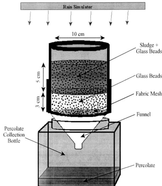
**FIGURE 1. Schematic of sludge incubation/leaching column.**
