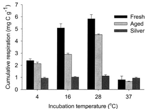
FIGURE 2. Microbial respiration results for fresh sludge, aged sludge, and silver biocide-treated sludge.
