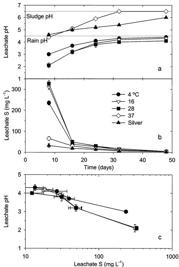
FIGURE 3. Temporal trends in leachate pH (a) and leachate total S (b), and the correlation between leachate pH and S (c). Dotted lines in panel a denote initial sludge pH and the input synthetic acid rain pH.
