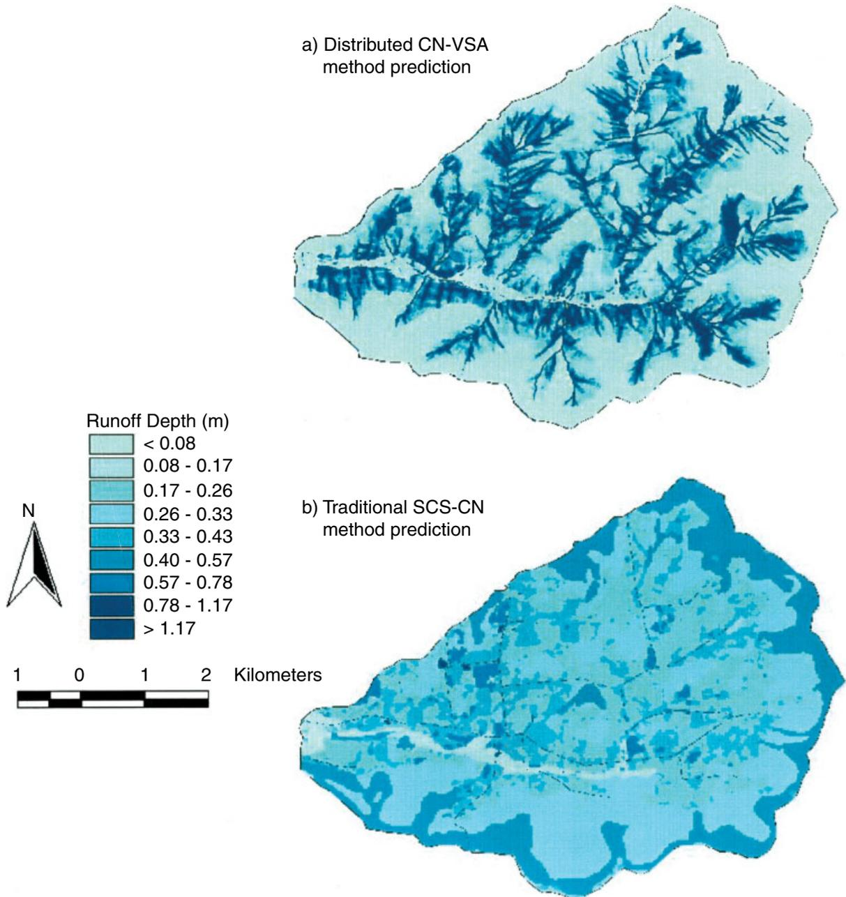
Figure 7. Total runoff depths for all summer events for Town Brook watershed using (a) the distributed CN–VSA method and (b) the traditional SCS-CN method
