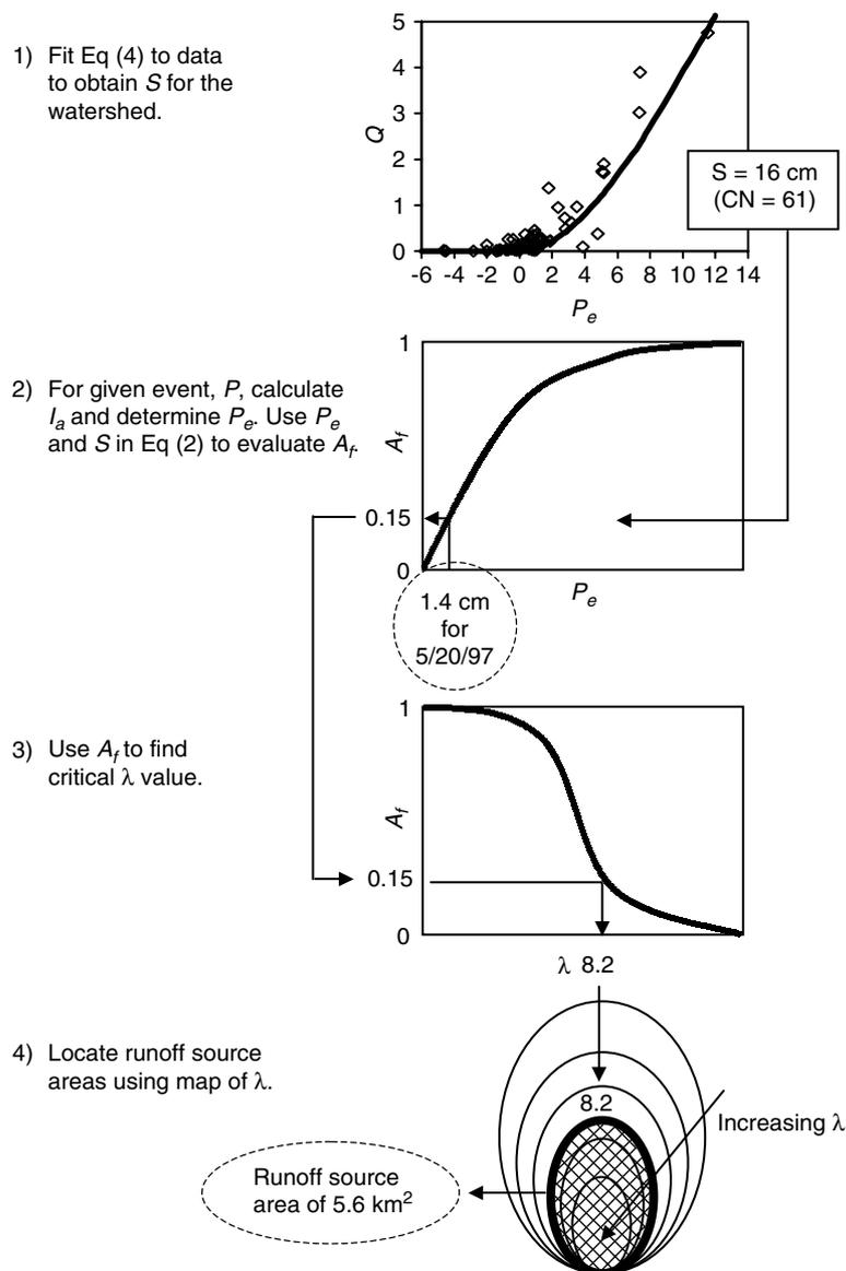
Figure 1. Overview of the distributed CN-VSA method from obtaining  $S$  to distributing runoff generation (saturation) showing example calculation for Town Brook watershed on 20 May 1997 described in text
