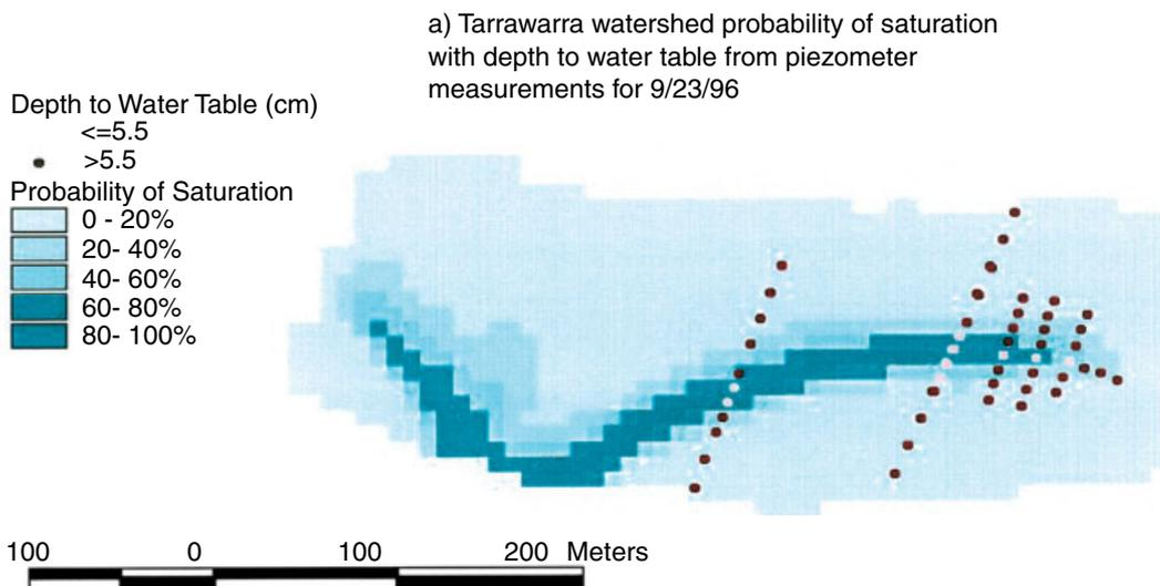
Figure 4. (a) Probability of saturation prediction using the distributed CN-VSA method with depth to water table measurements
