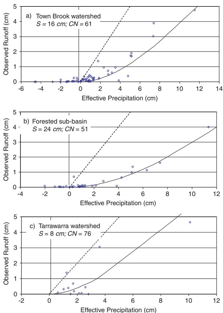
Figure 2. Calculation of  $S$  from observed runoff and effective precipitation using the method outlined by Steenhuis *et al.* (1995) for (a) Town Brook watershed, (b) forested sub-basin of Town Brook watershed and (c) Tarrawarra watershed
