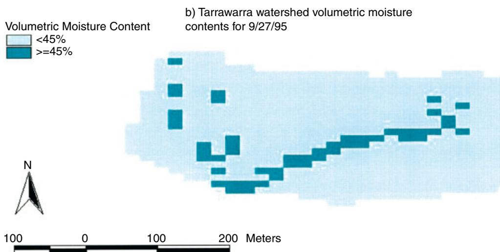
Figure 4. (b) Volumetric moisture content distribution using a TDR probe for the Tarrawarra watershed
