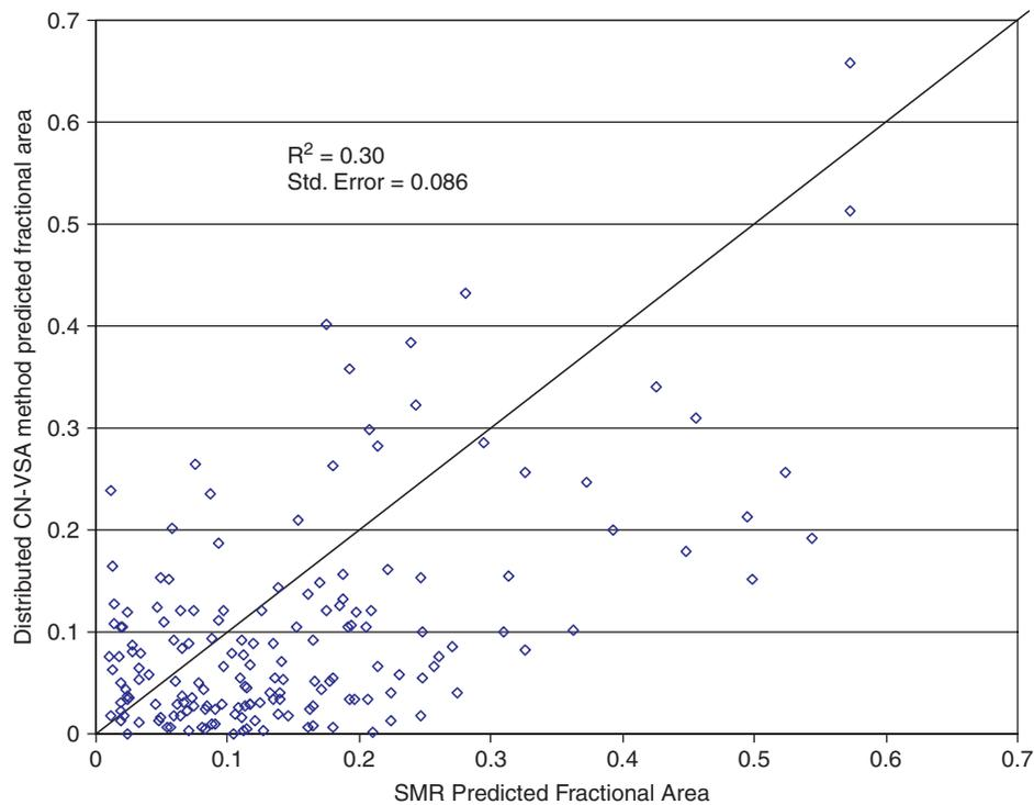
Figure 6. Fractional area of watershed saturating for summer  $P_e$  events predicted by the distributed CN-VSA compared with the SMR model prediction of fractional area of watershed for Town Brook watershed
