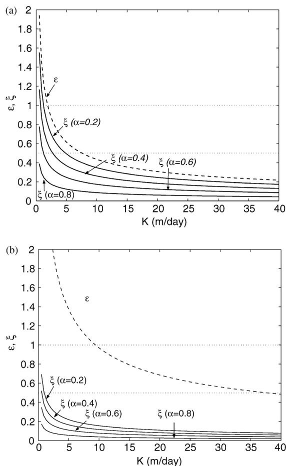
Fig. 2. Distribution of the shallow-water parameter ( $\varepsilon$ ) and steepness parameter ( $\xi$ ) versus hydraulic conductivity ( $K$ ) (a)  $D=1$  m and (b)  $D=5$  m.
