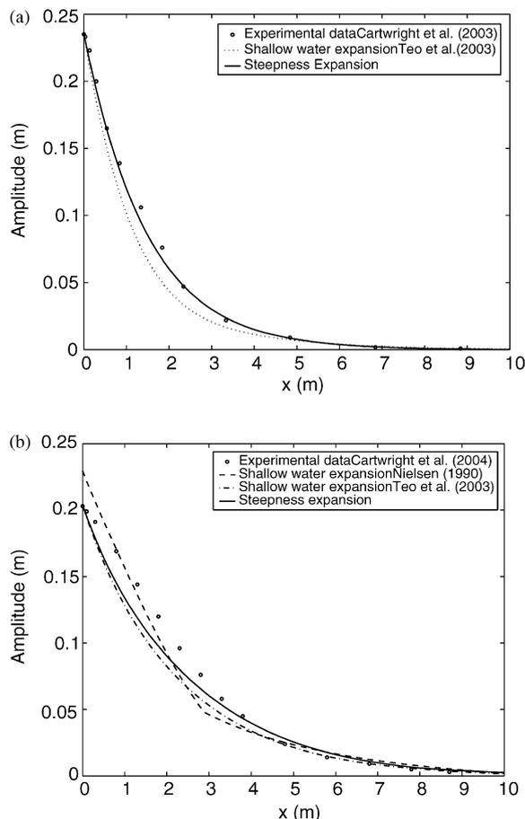
Fig. 3. Comparison of the two models against experimental data in (a) a vertical beach and (b) a sloping beach.
