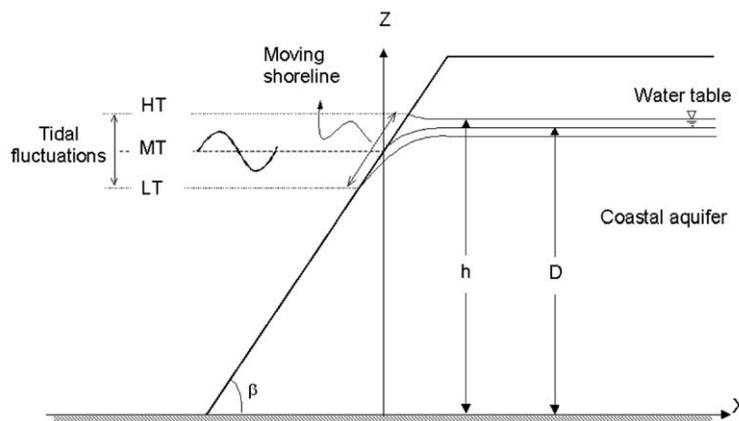
Fig. 1. Schematic diagram of tidal water table fluctuations in a coastal aquifer.
