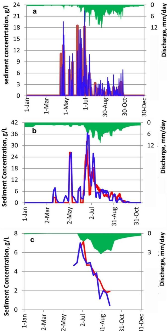
Figure 2: Predicted (red line) and observed (blue line) sediment concentration for a) Anjeni validation for daily concentrations in 1992; b) Enkulal calibration running weekly average concentrations in 2010; c) Validation for the Blue Nile at the Ethiopian-Sudan border in 2003. Discharge expressed in mm/day is the solid green area chart hanging from the top of figure
