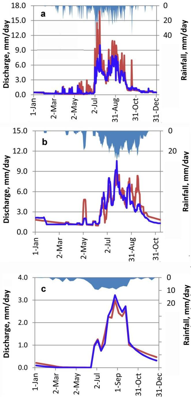
**Figure 1. Predicted (red line) and observed (blue line) discharge data for a) Anjeni validation for daily discharge in 1989; b) Enkual calibration running weekly average discharge in 2010; c) Validation for the Blue Nile at the Ethiopian-Sudan border in 2003.**
