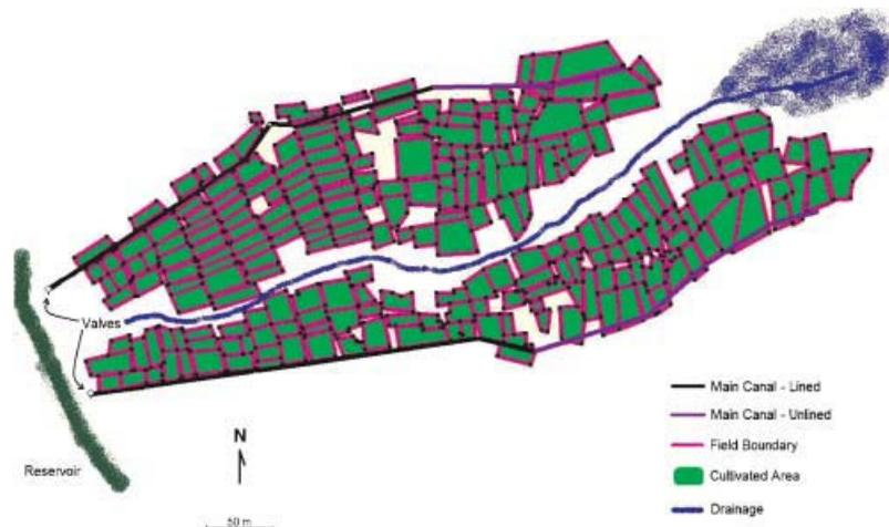
Figure 3. Weega system layout. This figure is available in colour online at [www.interscience.wiley.com/journal/ird](http://www.interscience.wiley.com/journal/ird)
