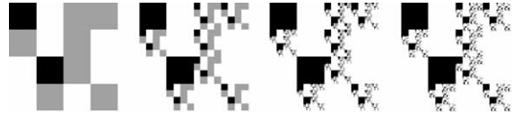
Fig. 2. Concept of the pore-solid fractal model for the first three iterations. The initiator is divided into matrix (white), pores (black) and an undefined set shown in grey. For each iteration step only the grey subregions are replaced by the initiator. Modified from Perrier et al. (1999).
