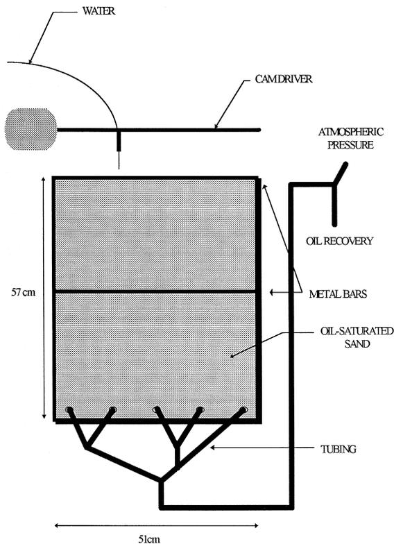
Fig. 2. Experimental chamber.
