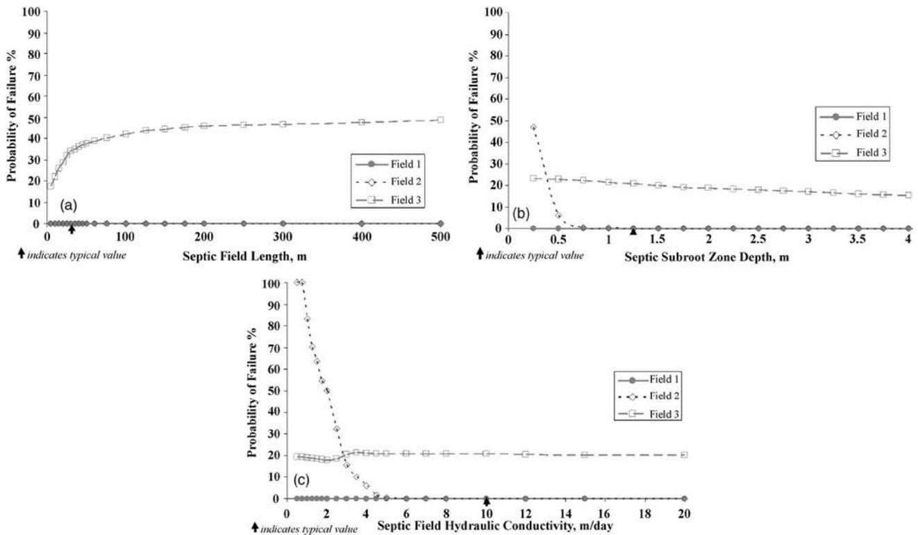
**Fig. 5.** Probability of failure in Fields 2 and 3 as a consequence of decreasing the conductivity in the septic effluent disposal field. Failure is defined for septic effluent disposal field (Field 2) when the water table exceeds the porous drain pipes and for Field 3 when the water table is within 20 cm of the surface. The water table height in Field 1 is not affected.
