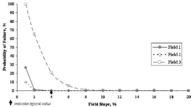
**Fig. 3.** Probability of failure in Fields 1, 2, and 3 as a consequence of varying the slope uniformly for all three fields. Failure is defined for Fields 1 and 3 when the water table is within 20 cm of the surface and for septic effluent disposal field (Field 2) when the water table exceeds the porous drain pipes.
