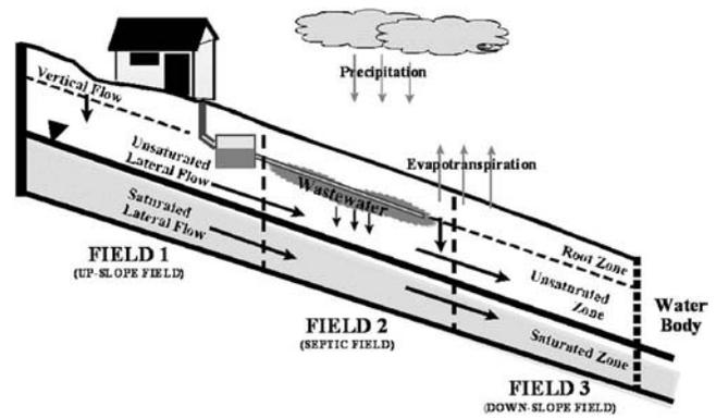
**Fig. 1.** Schematic drawing of the septic system being studied. From upslope to downslope: Field 1=upslope area; Field 2=septic effluent disposal field; Field 3=downslope area
