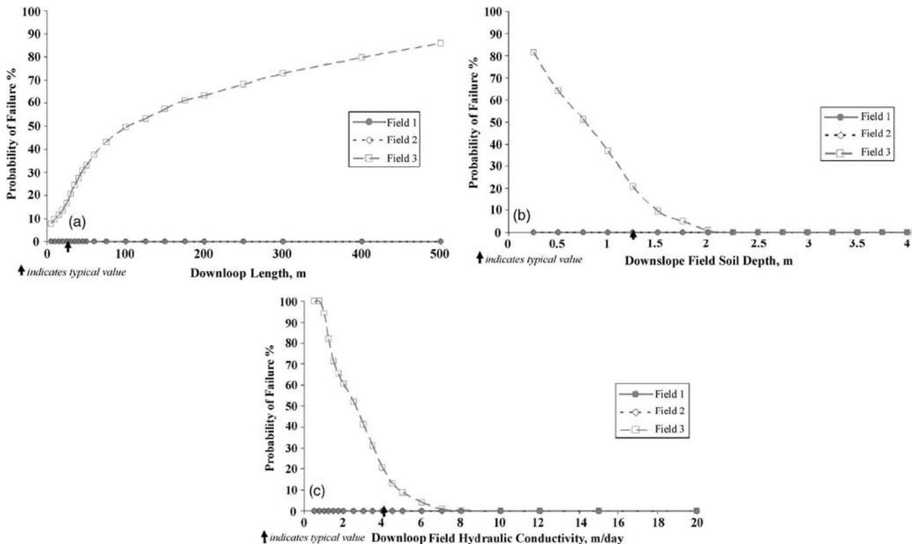
**Fig. 6.** Probability of failure in Field 3 as a consequence of changing the properties in Field 3. Failure is defined when the water table is within 20 cm of the surface: (a) downslope field length is varied; (b) downslope field subroot zone depth is varied; (c) downslope field saturated hydraulic conductivity is varied. The water table heights in Fields 1 and 2 are not affected.
