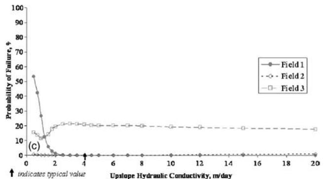
**Fig. 4.** Probability of failure in Fields 1, 2, and 3 as a consequence of changing the properties in Field 1. Failure is defined for Fields 1 and 3 when the water table is within 20 cm of the surface and for septic effluent disposal field (Field 2) when the water table exceeds the porous drain pipes: (a) upslope field length is varied; (b) upslope field soil depth is varied; (c) upslope field saturated hydraulic conductivity is varied.
