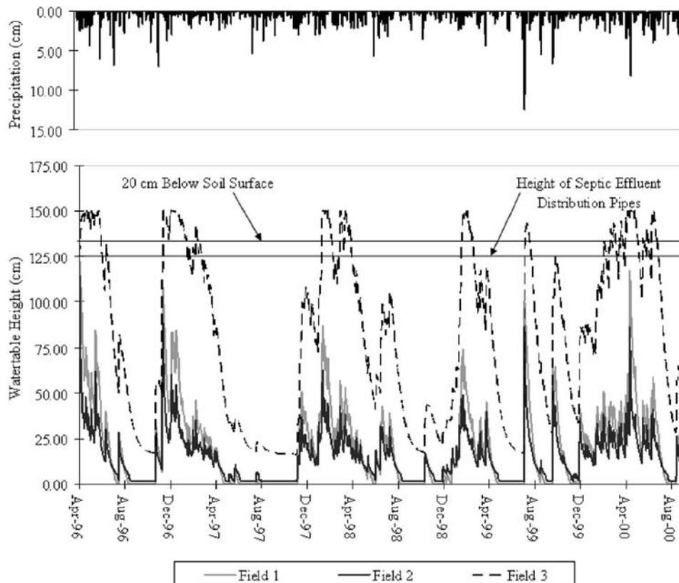
**Fig. 2.** Precipitation and simulated water table height for Fields 1, 2, and 3 for the period of April 1996 to August 2000
