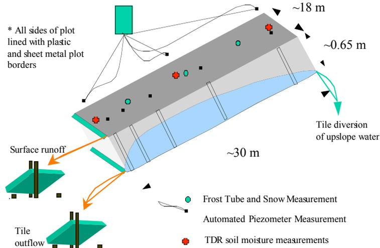
Figure 1 Hillslope plot layout and instrumentation.
