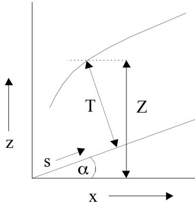
Figure 3. Conceptual model of lateral saturated flow to a tile (Childs, 1971).
