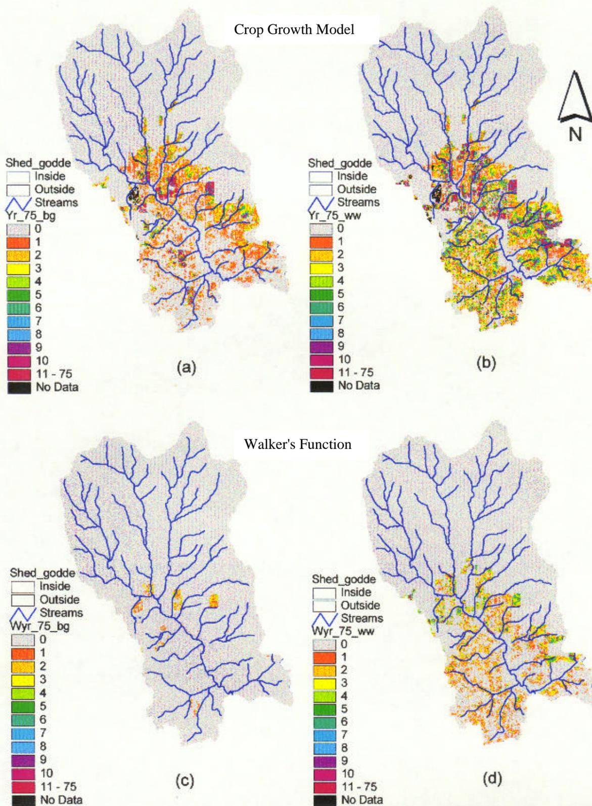
Figure 7. Yield Reduction after 75 Years of Onsite Erosion for Scenario 1 (left) and Scenario 2 (right).
