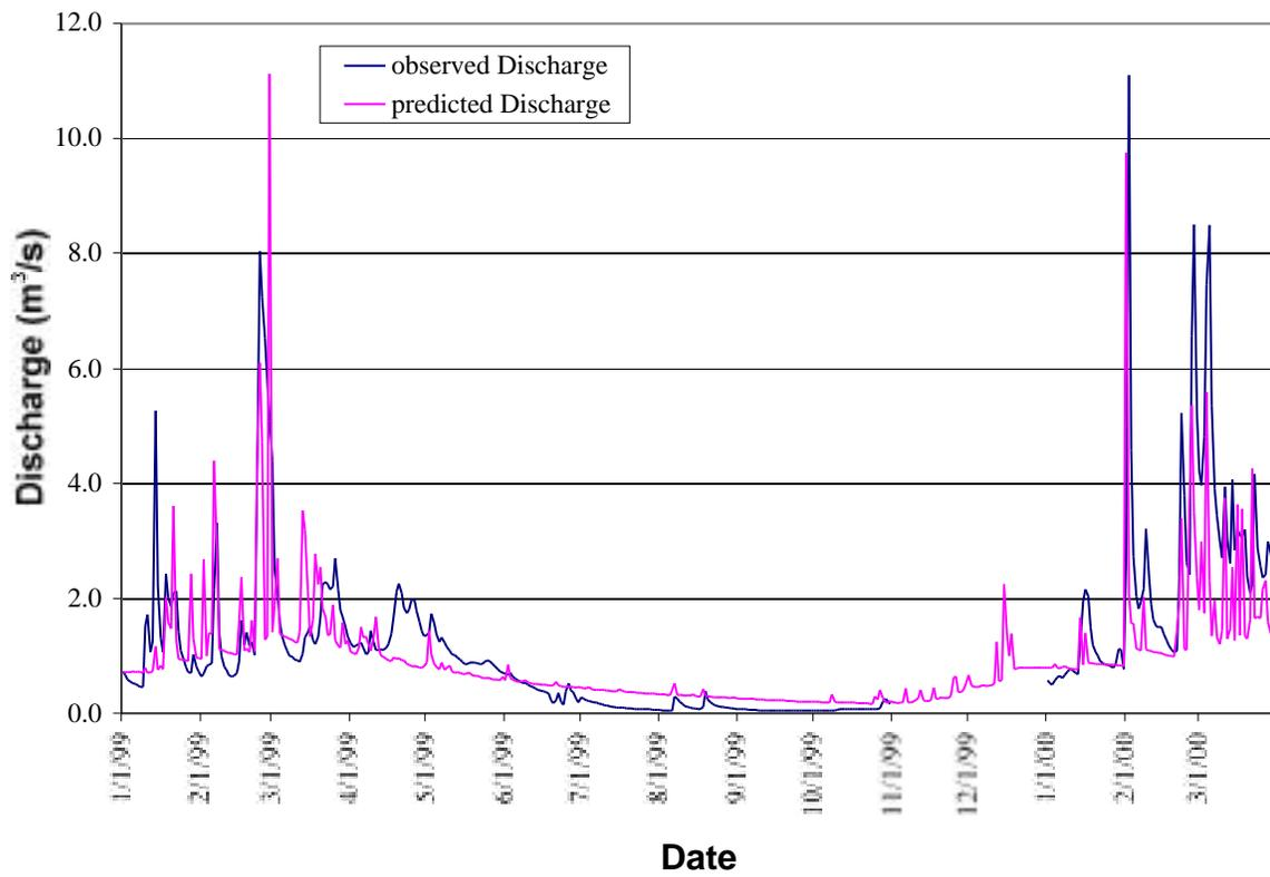
Figure 4. Observed and Predicted Stream Flow at Lower Monitoring Station in Lake Creek Watershed from January, 1999 to March, 2000.
