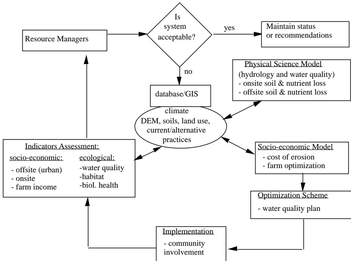
Figure 1. Schematic Representation of the GIS-based Integrated Systems Approach.
