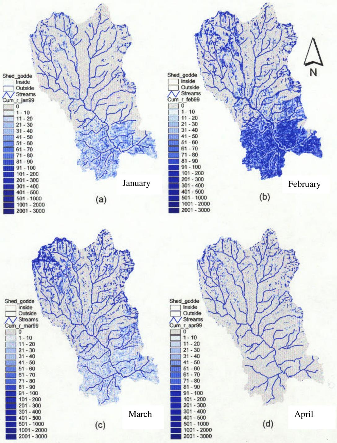
Figure 5. Cumulative Monthly Runoff (mm) for January (a) to April (d), 1999 in Lake Creek Watershed.
