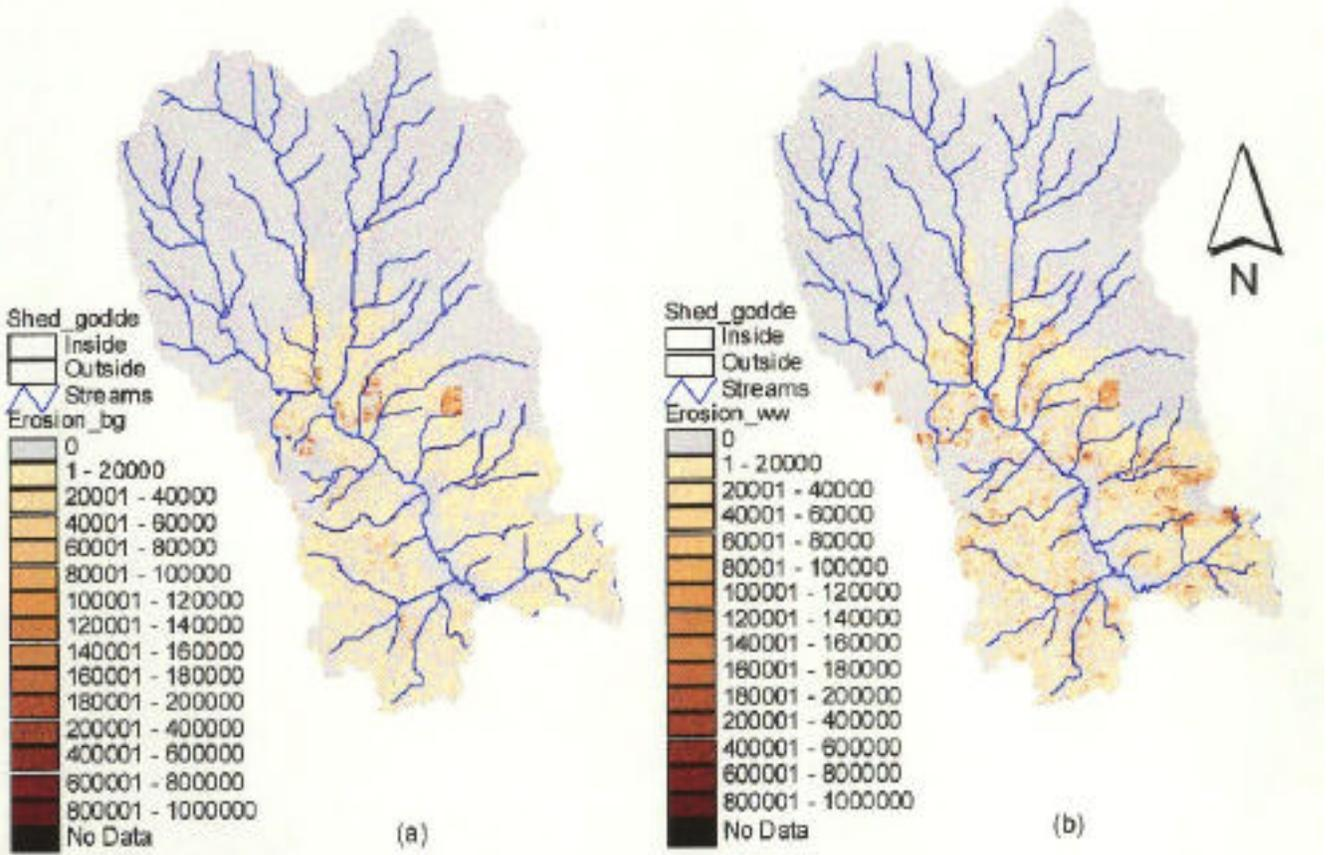
Figure 6. Erosion Prediction (Kg/ha) in Lake Creek Watershed for Scenario 1 (left) and Scenario 2 (right).
